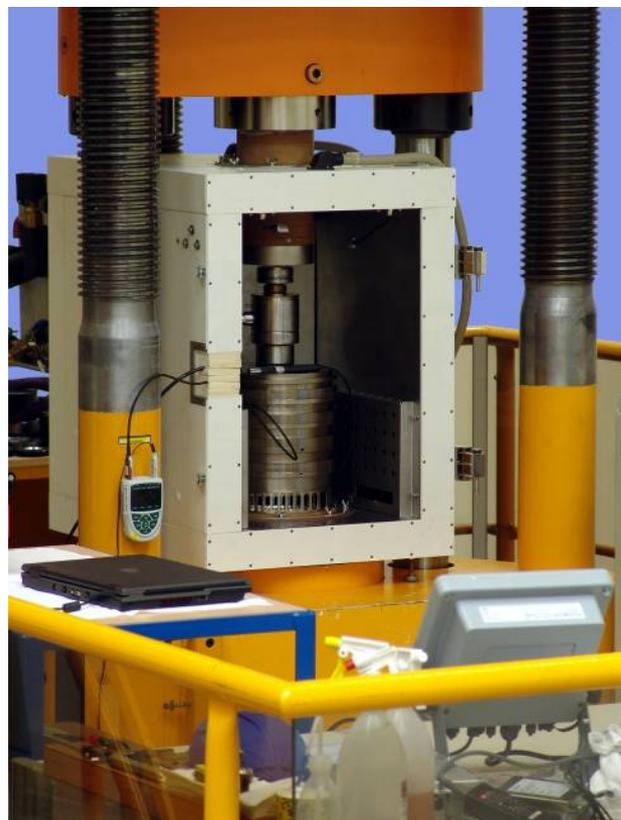
Figure 2. Example of an air-conditioned chamber integrated into a setup of a force calibration facility.
