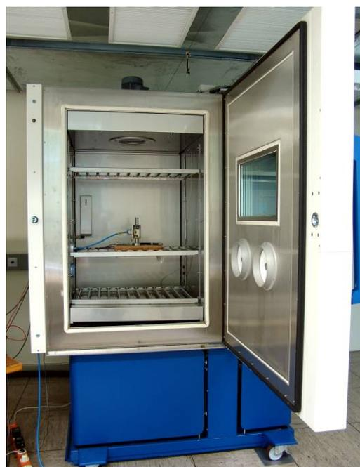
Figure 4. Ex-situ humidification of a torque transducer in a climate cabinet.
