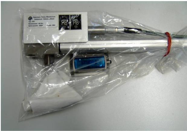
Figure 6. Ex-situ humidification of a torque wrench in a bag.
