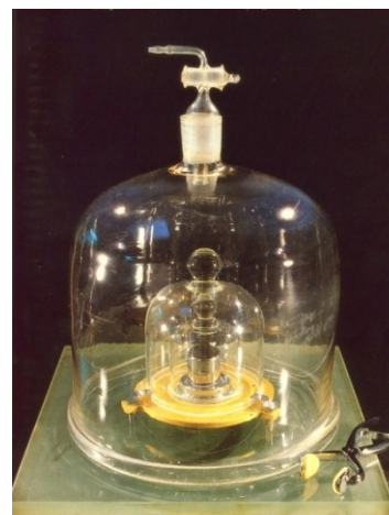
Figure 3. The IPK is kept at the BIPM in Sèvres. It still defines the unit of mass, the kilogram. Its mass, m_{\text{IPK}} , is defined to be exactly 1 kg with zero uncertainty. In the proposed new SI it will have non-zero uncertainty (source: BIPM, Sèvres, France).
