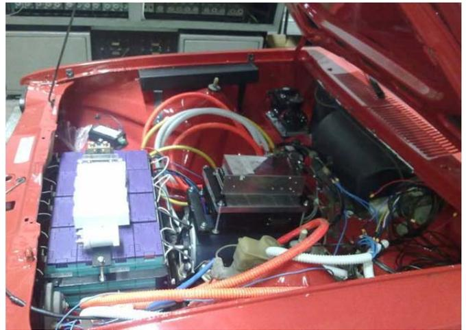
Figure 4. Battery pack in front of the induction motor.
