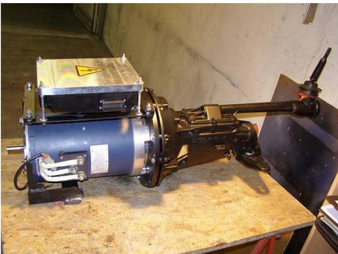
Figure 3. Induction motor with gearbox.
