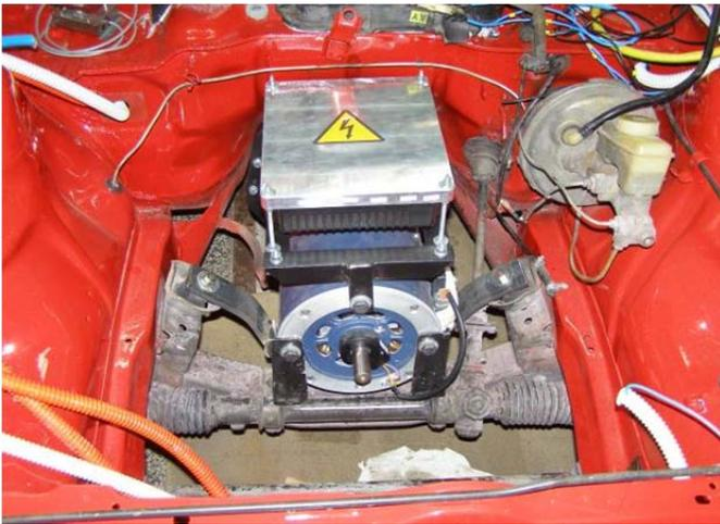
Figure 2. Induction motor with frequency converter installed in the vehicle.
