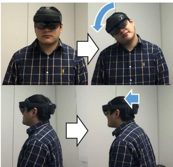
Figure 15. Top: Switch to posture instruction; Bottom: Switch to position instruction.
