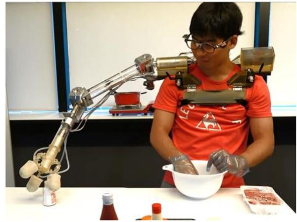
Figure 2. External view of the robotic arm proposed by Nakabayashi et al. [14] and Amano et al. [16].
