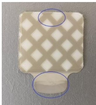
Figure 6. Area of the electrode for measuring the resistance.
