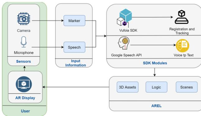
Figure 2. Architecture of the AREL System.
