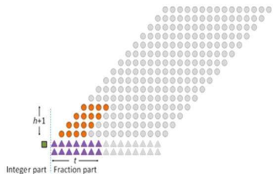
Figure 3. Representation of measured term  $1 + (Y_A)_t + (Y_B)_t + (Y_A)_{APX} + (Y_B)_{APX}$  in dot diagram with truncation 't' and rounding parameters 'h' are 7 and 3 respectively.
