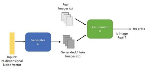
Figure 1. Flowchart for working of a GAN [3].
