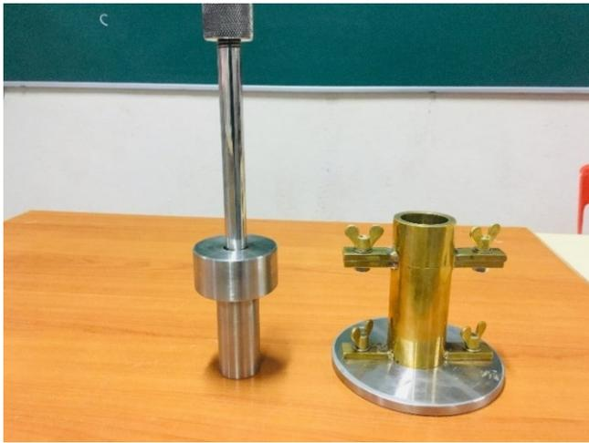
Figure 2. Mini compaction test apparatus.
