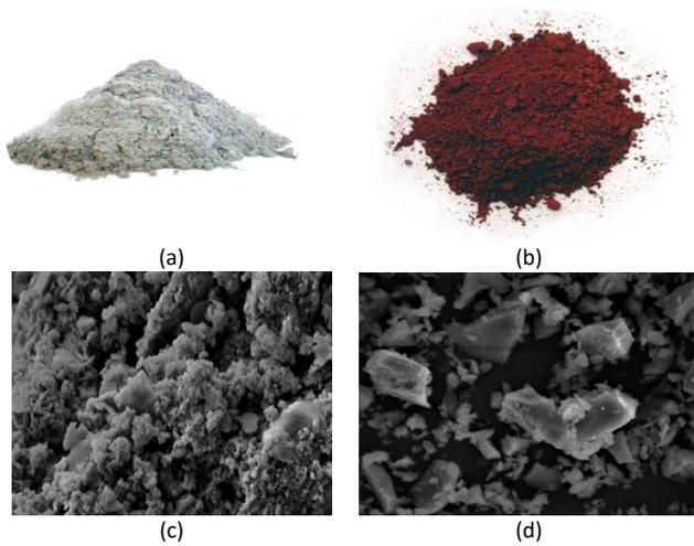
Figure 1. a) Original image of Red mud b) Original image of GGBS c) SEM image of Red mud d) SEM image of GGBS.
