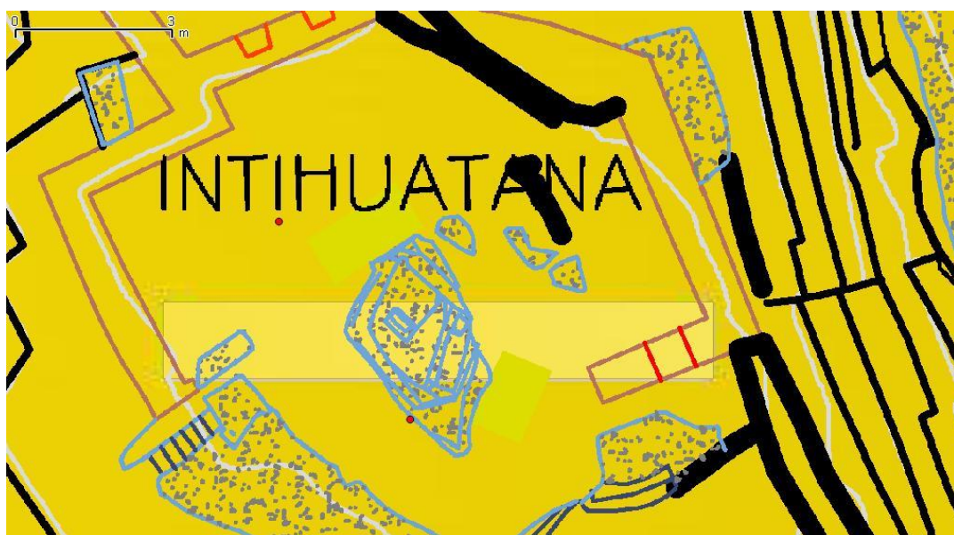
Figure 8. GNSS surveyed points (red) over 1:750 existing map.
