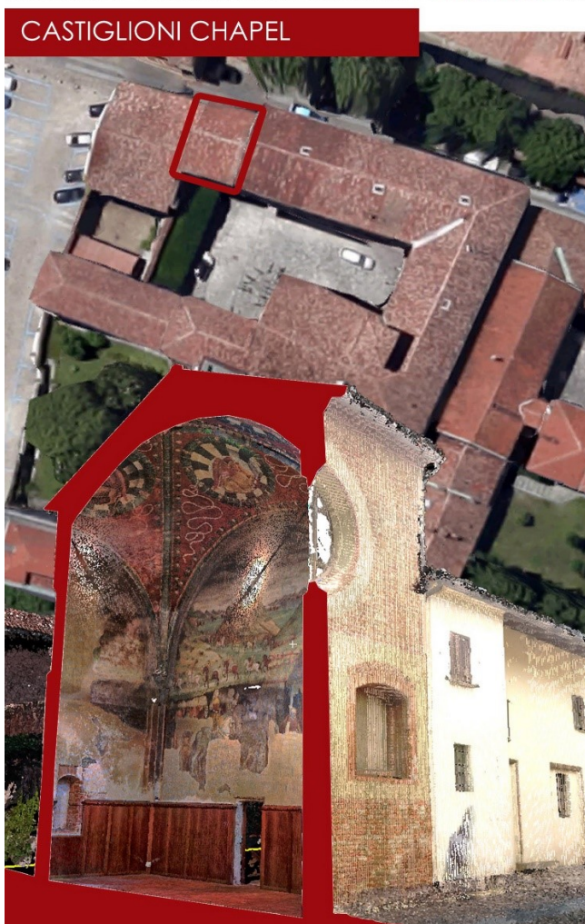
Figure 1. Setting of the College in Pavia city centre and a section of Castiglioni Chapel made by TLS point cloud.
