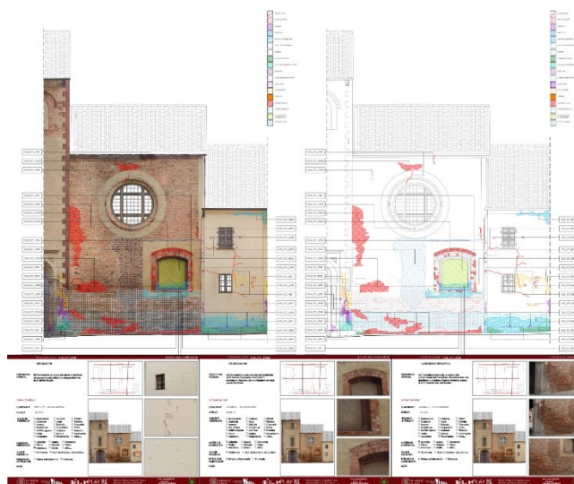
Figure 6. The integrated laser scanner and UAV survey made it possible to fully acquire the internal and external surfaces of the chapel.
