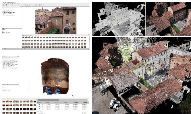
Figure 6. The integrated laser scanner and UAV survey made it possible to fully acquire the internal and external surfaces of the chapel.
