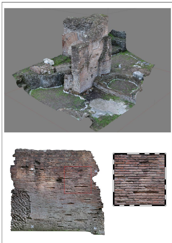
Fig. 6. Digital photogrammetry of ancient walls
