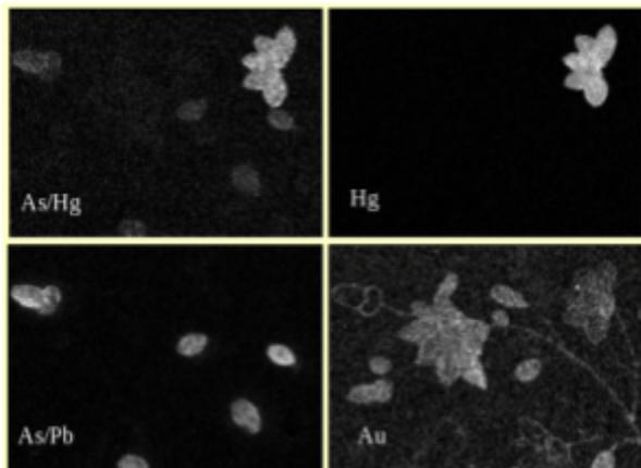
Fig.6 Elemental maps at 11.7 keV (As/Hg), 9.9 keV (Hg), 10.5 keV (As/Pb) 9.6 keV (Au). The scanned is 14,5 10,5 cm<sup>2</sup>.
