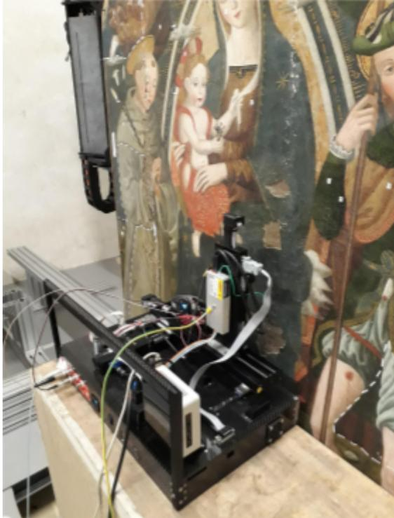
*Fig.1 INFN-CHNet MA-XRF scanner positioned in front of a panel on canvas at the CCR La Venaria Reale.*
