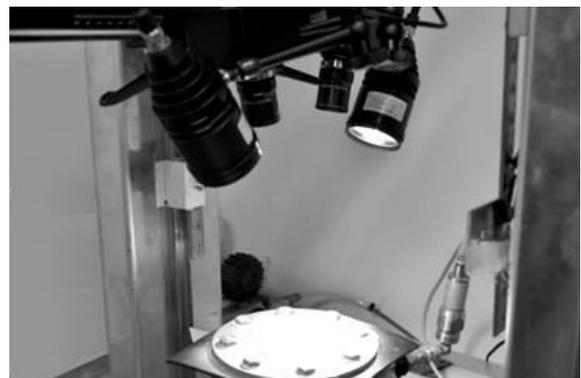
Figure 3. Bulge test setup for 3D-DIC technique (Courtesy of authors [22]).
