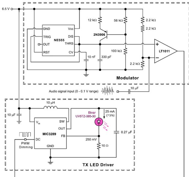
Figure 12. Audio modulator and LED driver.
