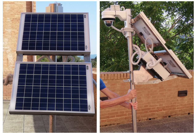
Fig. 2. Realization of the video monitoring system: photovoltaic panels (left) and pole with camera and IP56 box containing the electronics (right).
