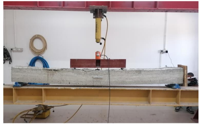
Figure 6. Experimental setup for post-mechanical tests on the beam.
