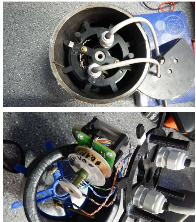
Fig. 3. The fully equipped laboratory ME sensor intended for the experiment on the patent wire P7, the assembled sensor inside the steel shield (above) and view on its disassembled basic parts (below)
