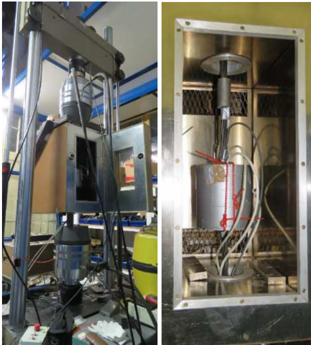
Fig. 4. The exterior view on the climatic chamber and the steel tensile testing machine (on left) and on the laboratory ME sensor installed on the prestressed strand Lp15.7 inside the chamber (on right)
