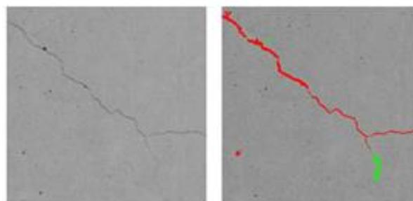
Figure 1. Digital image processing of concrete wall surface image showing crack.
