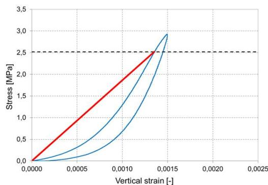
Figure 19. Stress vs. strain curve obtained by contact dimensional measurement.
