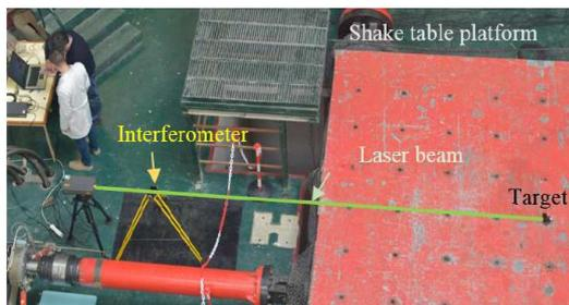
Figure 11. Experimental setup for rotation motion testing.
