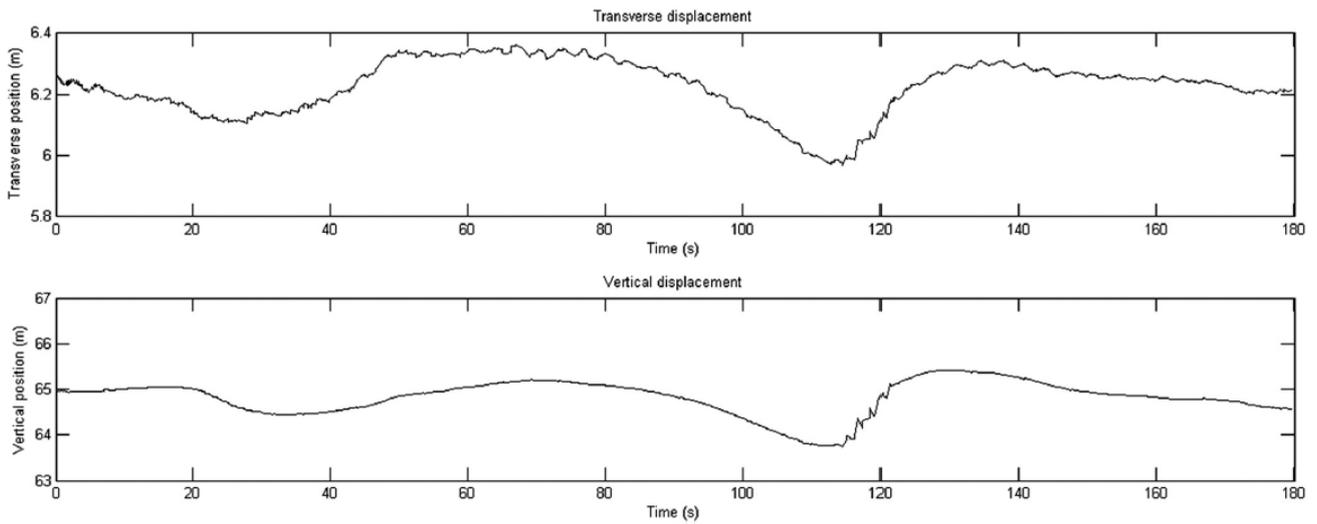
Figure 4. P25A main span central section displacement - train and road traffic.
