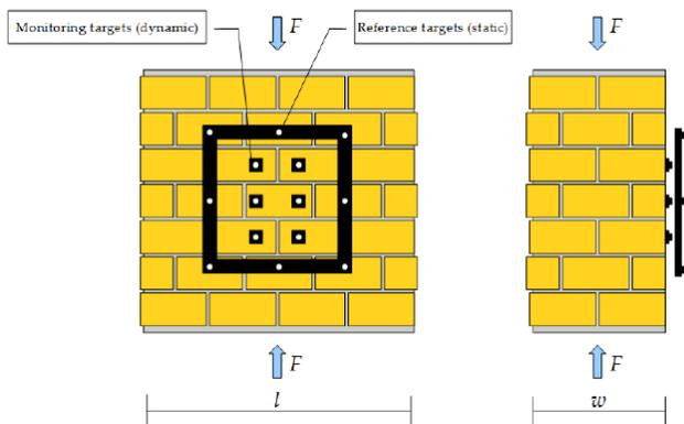
Figure 15. Schematic representation of the proposed optical measurement method.
