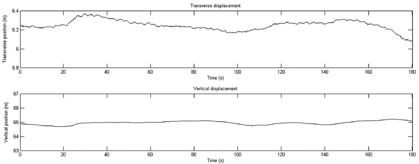
Figure 5. P25A main span central section displacement - road traffic only.
