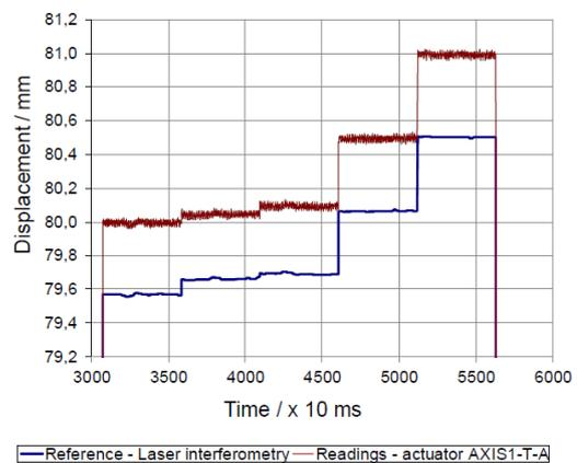
Figure 14. Results of the discrimination test of axis 1-T-A at the 80 mm position.
