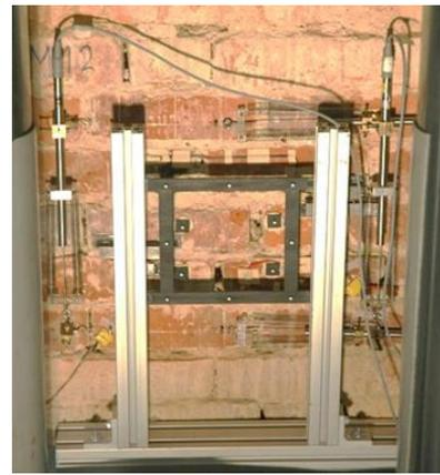
Figure 16. Instrumentation of the masonry specimen.
