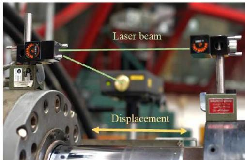
Figure 10. Experimental setup for cross-axis motion testing.
