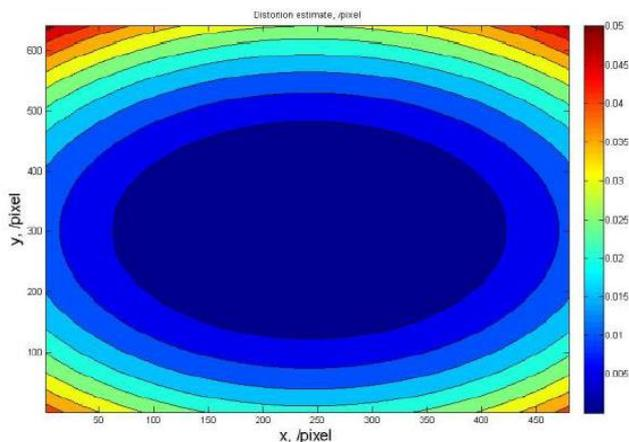
Figure 7. Image distortion estimates in pixels.
