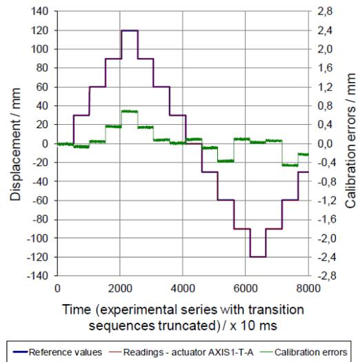
Figure 13. Calibration errors for the dynamic position test of axis 1-T-A.
