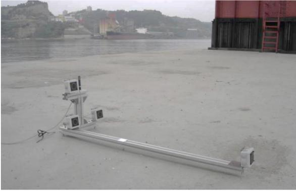
Figure 2. Active targets on the south tower foundation.
