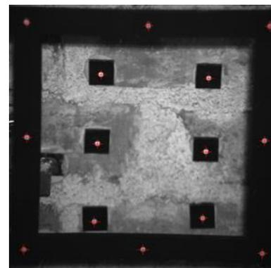
Figure 17. Example of targets image after digital processing, showing the determined centroids.
