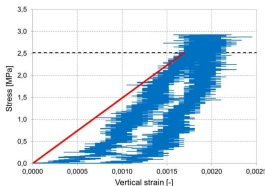
Figure 20. Stress vs. strain curve obtained by optical dimensional measurement.
