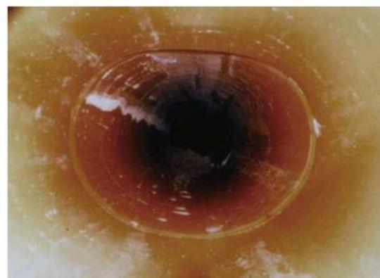
Figure 6. Inspection image showing dimensional reduction by deformation effect [13].
