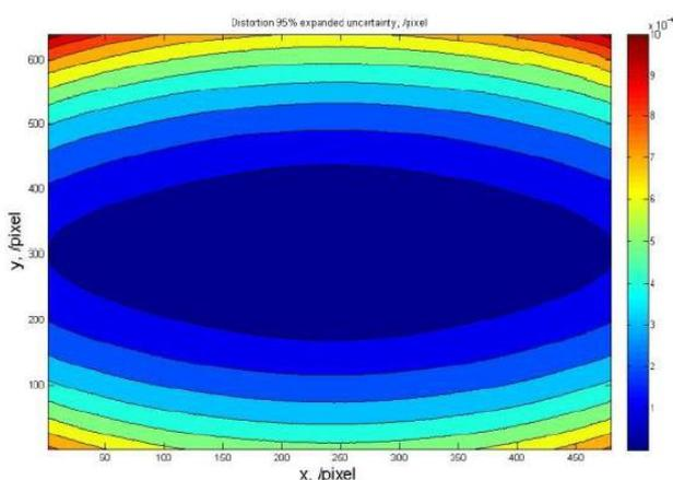
Figure 8. Image distortion 95 % expanded uncertainties in pixels.
