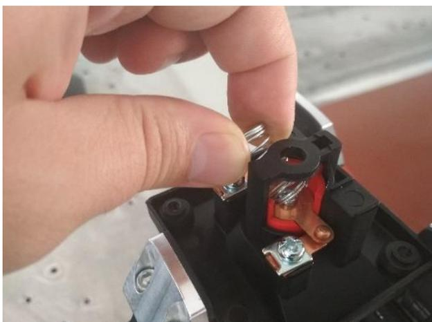
Fig. 2. Illustration of a manual spring insertion.
