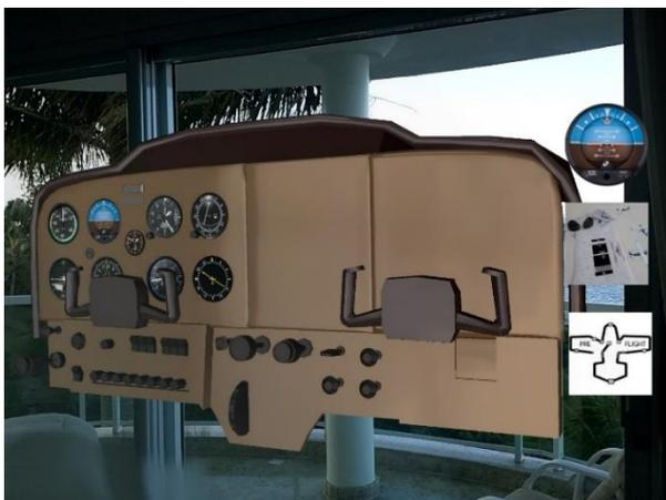
Figure 2. A life-size panel that can be viewed at home using a smartphone and a banner printed marker.
