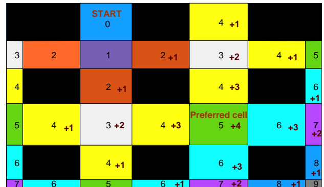
Fig. 3: Distance values and additional preference values when applying additional preference (value of 4 and range of 4), normal numbers represent the distance values, bold numbers represent the additional preference values
