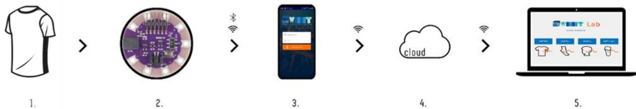
Figure 1. System architecture: 1) wearable sensing device, 2) electronic unit, 3) SWEET App, 4) cloud, 5) SWEET Lab.
