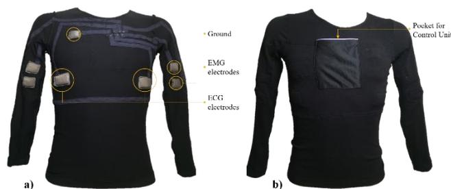
Figure 2. SWEET shirt sensing unit: a) internal view with textile electrodes and connections, b) external view.
