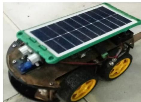
Figure 2. Assembled vehicle with the solar panel installed on the roof.
