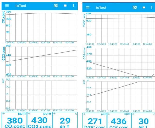
Figure 13. Screenshot of the IoTool application during experiments performed on the mobile robot's sensing system, showing the temporal trends of the interest parameters.
