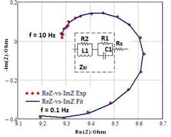
Fig. 6. Fitting result of LF part of data ( $f=10-0.1$  Hz). Nichrome wire at  $V_{dc}=5.3$  V:  $R_s=8.261 \Omega$ ;  $R_1=0.622 \Omega$ ;  $C_1=0.373$  F;  $R_2=1.018 \Omega$ ;  $L_1=1.091$  H
