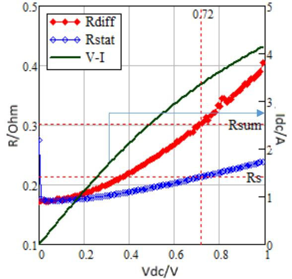
Fig.10. I-V – curve; static and differential resistance curves of silver wire with the same dimensions as in Fig. 2
