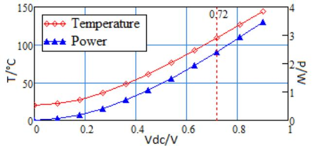
Fig. 8. Power dissipation and temperature of silver wire - refer to the experiment data in Fig. 2
