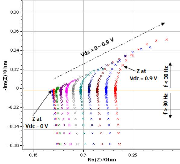
Fig. 2. Nyquist plot of silver wire at  $V_{dc}=0 - 0.9$  V with bias step  $0.09$  V; length  $500$  mm and diameter  $0.25$  mm
