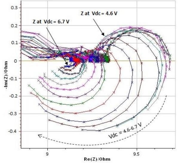
Fig. 3. Nyquist plot of nichrome wire at  $V_{dc}=4.6 - 6.7$  V with bias step  $0.1$  V; length  $57$  mm and diameter  $0.1$  mm
