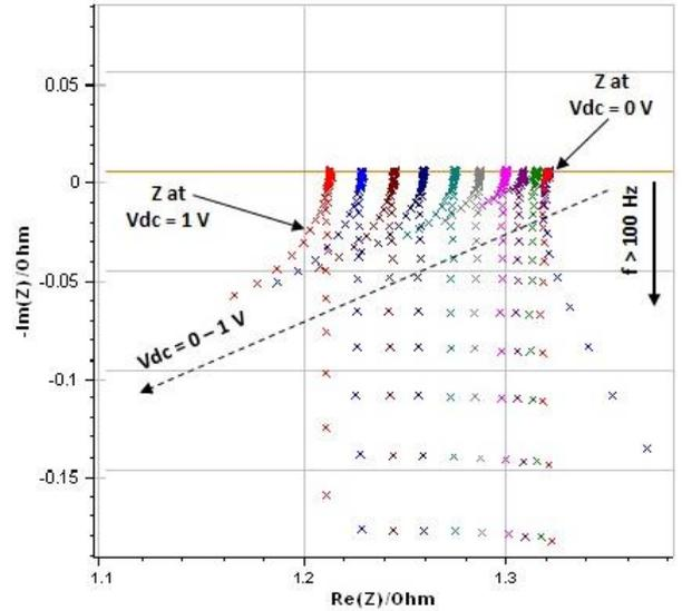
Fig. 4. Nyquist plot of graphite rod at  $V_{dc}=0 - 1$  V with bias step  $0.1$  V; length  $57$  mm and diameter  $0.5$  mm
