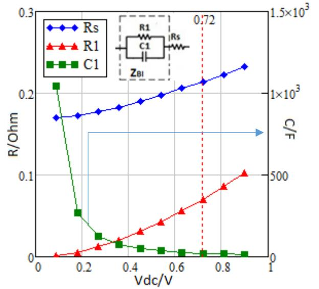
Fig. 7. Model parameters of silver wire as a function of bias - refer to the experiment data in Fig. 2
