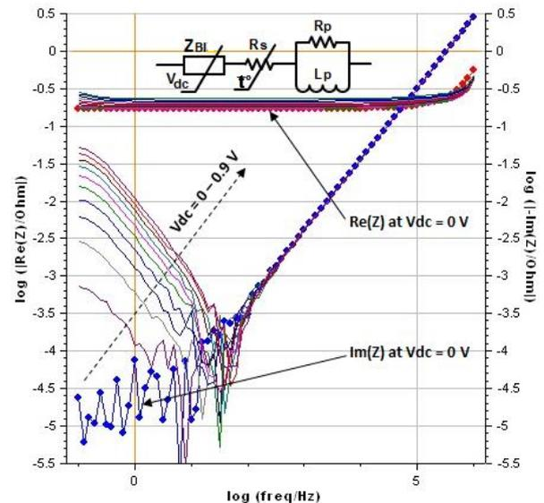
Fig. 1.  $Re(Z)$  and  $Im(Z)$  of the silver wire at  $V_{dc}=0 - 0.9$  V with bias step 0.09 V; length 500 mm and diameter 0.25 mm; frequency range 1 MHz - 0.1 Hz
