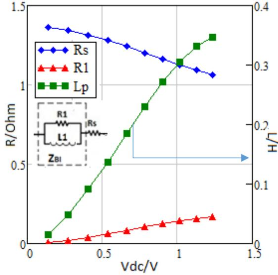
Fig. 9. Model parameters of graphite rod as a function of bias - refer to the experiment data in Fig. 4
