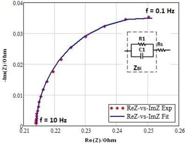
Fig. 5. Fitting result of LF part of data ( $f=10-0.1$  Hz). Silver wire at  $V_{dc}=0.72$  V. Fit parameters:  $R_s=0.214 \Omega$ ;  $R_1=0.07 \Omega$ ;  $C_1=21.34$  F
