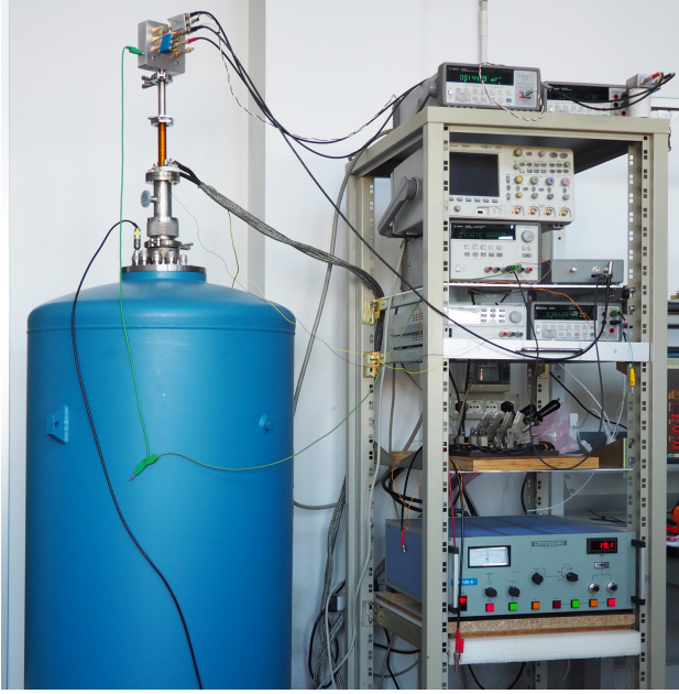
Fig. 7. Overall view of the measurement setup for DC characterisation. On the left, the liquid helium dewar, with the coaxial probe inserted. On the right, the rack of electronic instrumentation.
