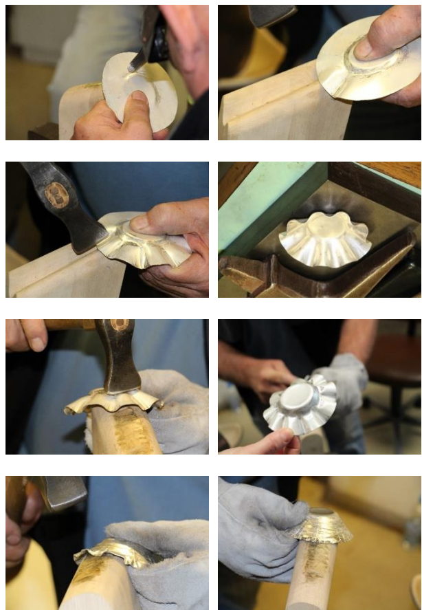
Fig.2. Initial steps of preparing wrinkling cup. Placing contours, wrinkles and hammering of wrinkles
