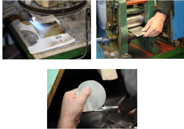
Fig.1. Annealing rolling and cutting the initial silver sheet.
