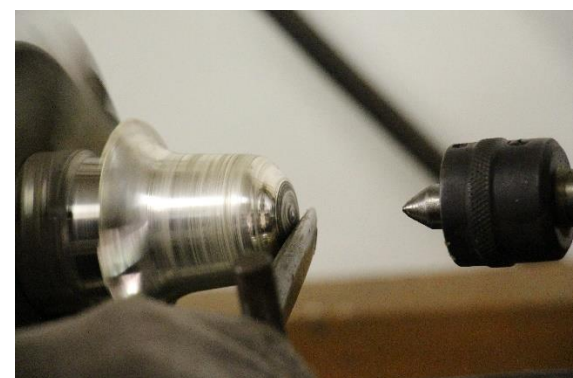
Fig.4. Subsequent steps of preparing metal spinning cup.
