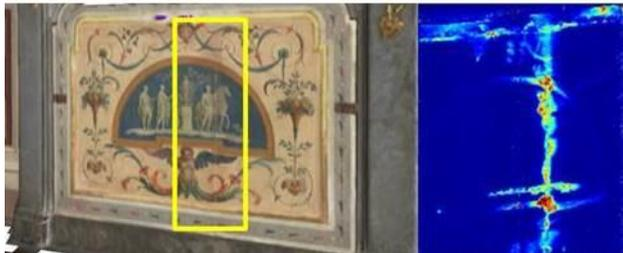
Figure 9. Top: RGB-ITR image with measured area in black line (left) and corresponding false colour LIF image (right). Bottom: Fire screen RGB-ITR image, with measured area in yellow line (left) and corresponding LIF 380/450 nm image (right).
