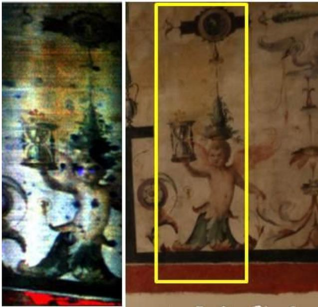
Figure 5. False colour LIF image reconstructed at 300, 400 and 500 nm on the left; photogrammetric image with measured area in the yellow line on the right.
