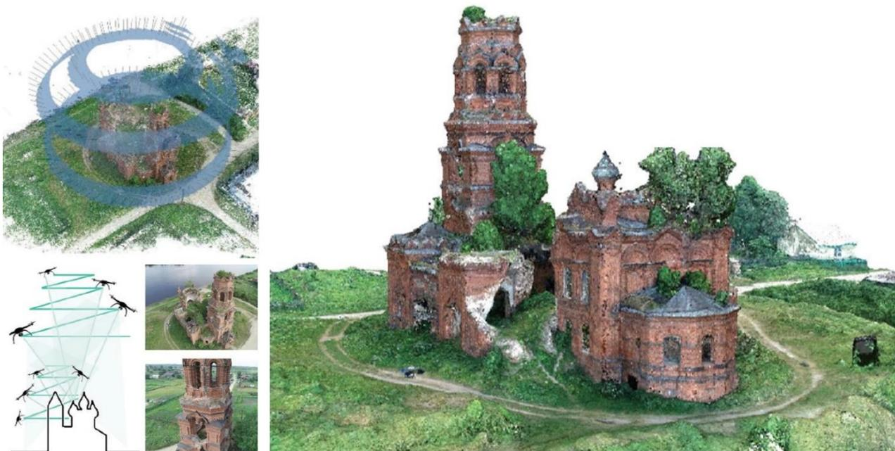
Figure 6. Morphometric database from the on-site photogrammetric UAV acquisition campaign: the photos were geo-referenced and aligned to define the main point cloud on the architectural complex and the surrounding landscape.
