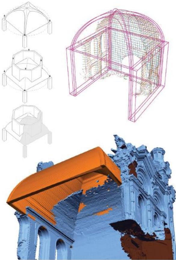
Figure 12. NURBS modelling of the pavilion vault from the sections extracted by the mesh surface. The geometric vault was referenced to the mesh model and was imported in the same workspace.
