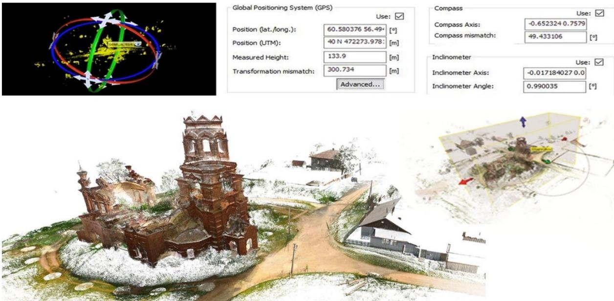
Figure 5. Morphometric database from on-site TLS acquisition campaign: the single scans, completed via GPS, compass, and inclinometer information, were referenced and registered to control the overall alignment to verify the final point cloud.
