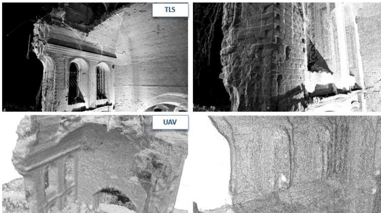
Figure 9. Quality of processed morpho-metric TLS and UAV data on the internal surfaces of the masonry structure. The point cloud from the UAV acquisition shows a worse resolution in the discrete definition of the main profiles, geometries, and surfaces, largely due to the corner and shadow shooting.
