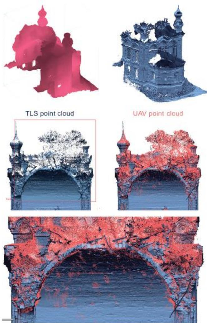
Figure 10. Alignment and integration of multi-instrumental point clouds for the static unit of the central pavilion vault.
