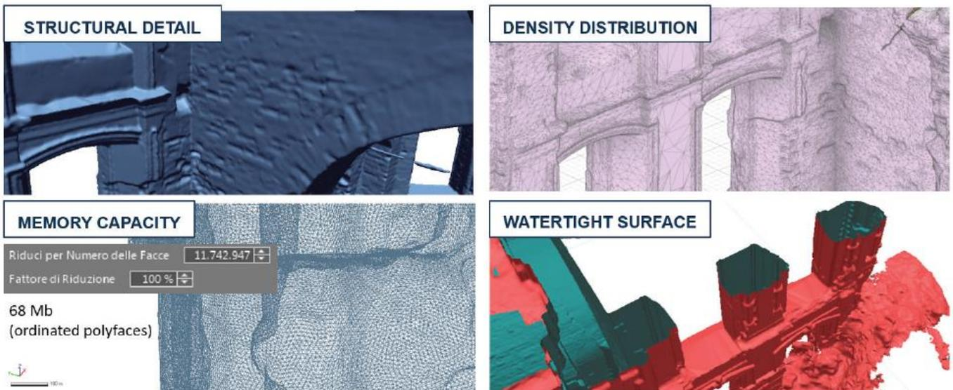
Figure 14. Properties of the final HD mesh model, which is suitable for compatible computing analysis in FEA workflows.
