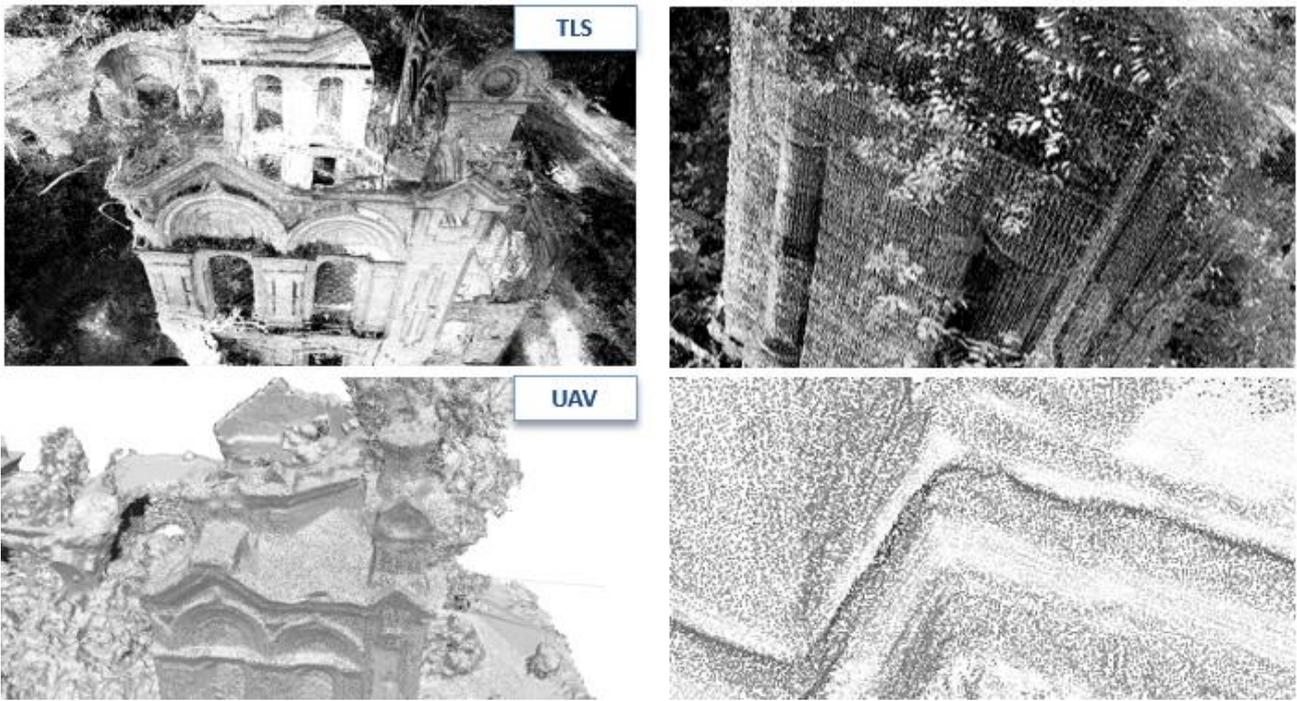
Figure 8. Quality of processed morpho-metric TLS and UAV data on the external surfaces of the masonry structure. The point cloud from the UAV acquisition shows a resolution and density of data comparable with the TLS acquisition, supported by the higher level and resolution of the camera shooting.
