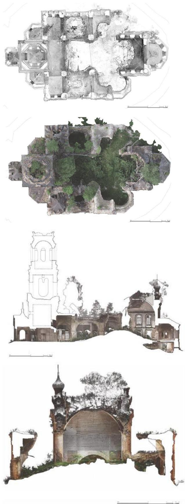
Figure 7. Drawings and elaborations for the 2D description of the main structural system of the church. The presence of noise data for elements such as the vegetation and collapsed ruins is highlighted.
