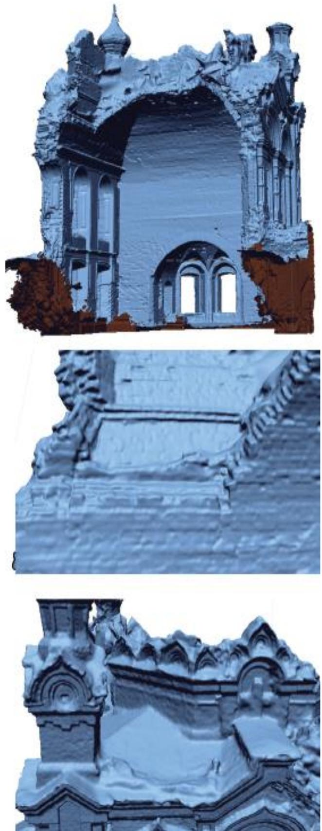
Figure 11. Final reality-based mesh models following the triangulation and optimisation processing of the HD mesh. The mesh preserved the specific details of the structural shape of the structural unit.
