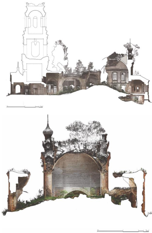
Fig. 3. Vectorial and metric sections of Blagoveshchenskaya Church and of the main ruin vaulted central environment
