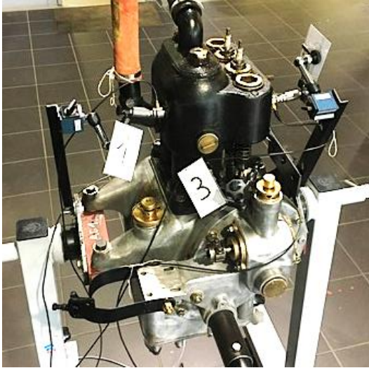
Fig. 2. AE sensors location on a Renault AG1 engine © MNAM, 2018
