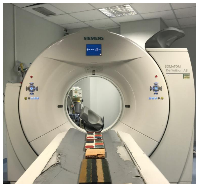
Figure 1. Wooden tablets painted with the most commonly used ancient pigments placed on the CT scanner bed for MSCT scanning.
