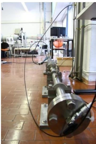
Figure 1: Developed diaphragmless shock tube with a quick-acting valve
