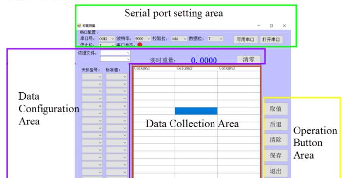
Figure 4 Automatic processing software interface
