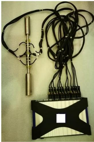
Figure 2: Alignment tool kit from ZwickRoell
