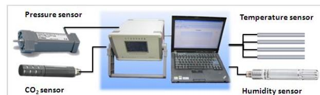
Figure 2: Pictures of air density measurement system
