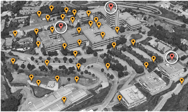
Fig. 7. The simulated scenario with 3 GWs located in the campus area: hot spots (yellow markers) and GWs (white circled red markers) placement.
