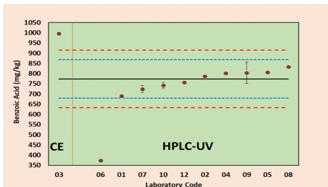
Figure 2. Participant results for MICPT-14-01: Benzoic acid in Mango Juice using capillary electrophoresis and high-performance liquid chromatography with UV detector.
