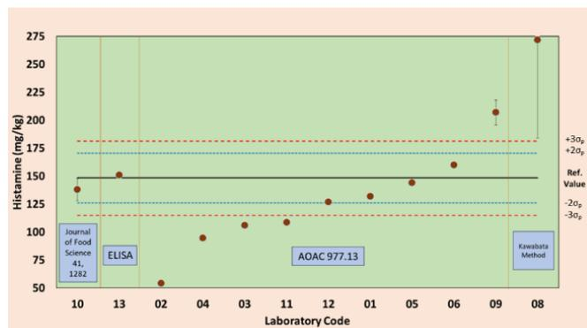
Figure 3. Participant results for MICPT-14-04: Histamine in canned tuna using fluorometer detection with different sample preparation.
