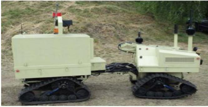
Figure 1. The demining UGV DROMADER.
