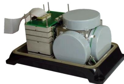
Figure 3. Navigation data from various types of sensors is fused directly onboard the 120/3 navigation system from Perm Instruments Making Company.
