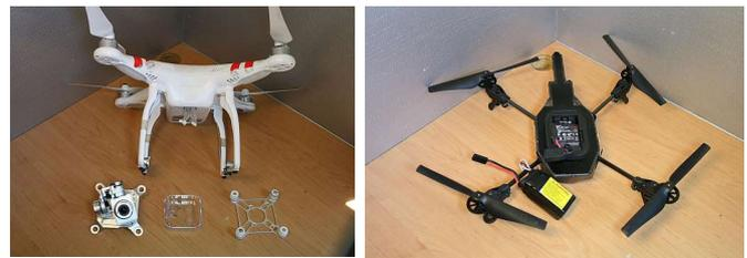
Figure 1. DJI Phantom 2 used as mothership UAV (left); Parrot AR Drone 2.0 used as child UAV (right).
