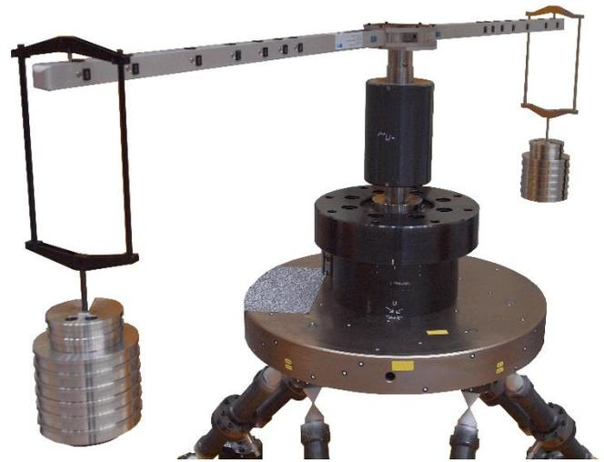
Figure 6. Lever/mass system and MCTT mounted in the measurement hexapod at PTB.
