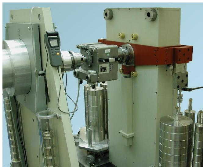
Figure 6. Mounting of the separate measurement module into a national torque standard machine of PTB for static torque calibration.
