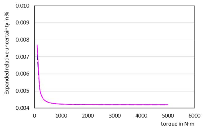
Figure 10. The confirmed uncertainty (solid pink line) and the expanded uncertainty (dash blue line) of the 5 kN·m torque standard.
