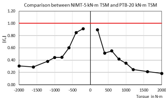
Figure 7. The  $|E_n|$  evaluated based on the comparison, ranging from 200 N·m to 2,000 N·m.
