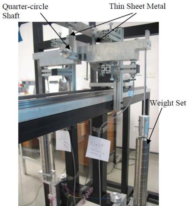
Figure 1. Suspended-Fulcrum Torque standard machine of NIMT (10-N·m-DWTSM).
