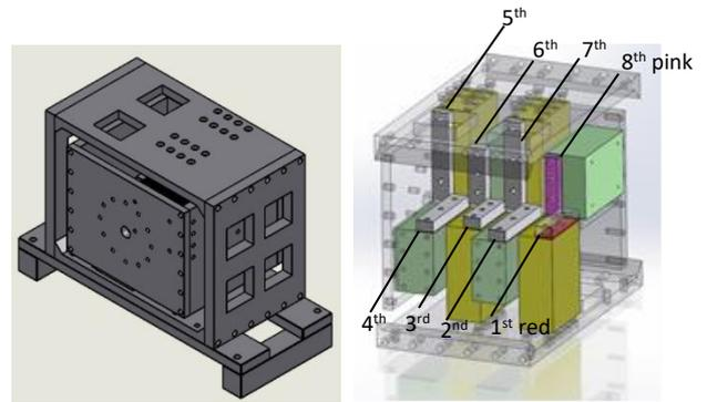
Figure 3. Schematic diagram of flexure bearing with eight elastic hinges (four pieces, highlighted in red, and four pieces highlighted in pink).
