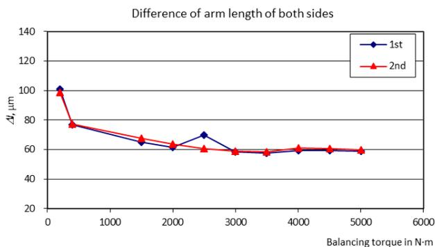
Figure 8. The difference in arm length ( $\Delta l$ ) of both sides of the machine. 1st represents the first series of the measurement. 2nd represents the second series of the measurement.
