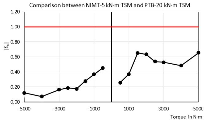
Figure 9. The  $|E_n|$  evaluated from the comparison, ranging from 500 N·m to 5,000 N·m.
