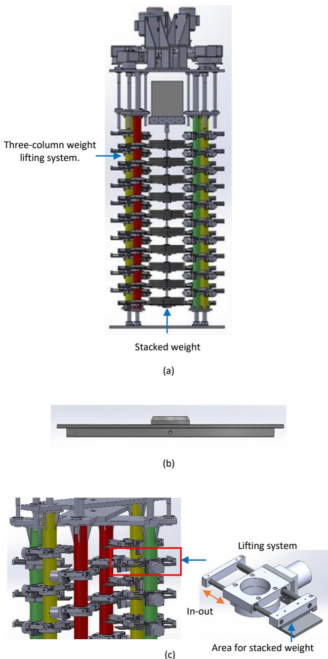
Figure 5. (a) A schematic overview of the stacked weight with the lifting system. (b) One piece of the weight disk. (c) Three-column (highlighted in red, yellow, and green columns) weightlifting system.
