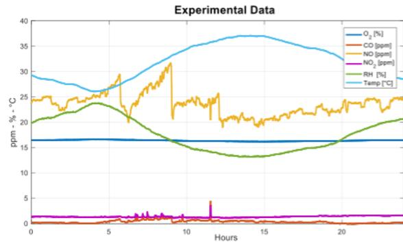
Fig. 5. Example of data obtained from the monitoring of a combustion process.
