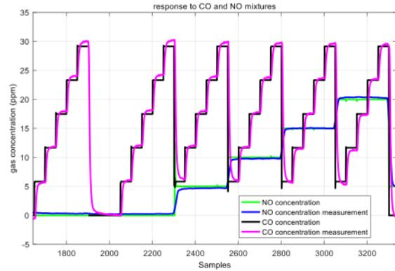
Fig. 4. CO and NO measurements obtained with NO and CO mixtures in air (RH = 50%, flow rate 200mL/min). The true concentration of the two gases are indicated with green and black lines.
