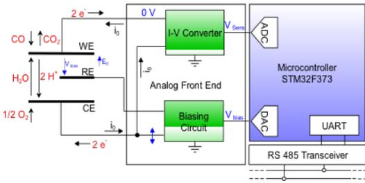
Fig. 3. Electrochemical front end structure.
