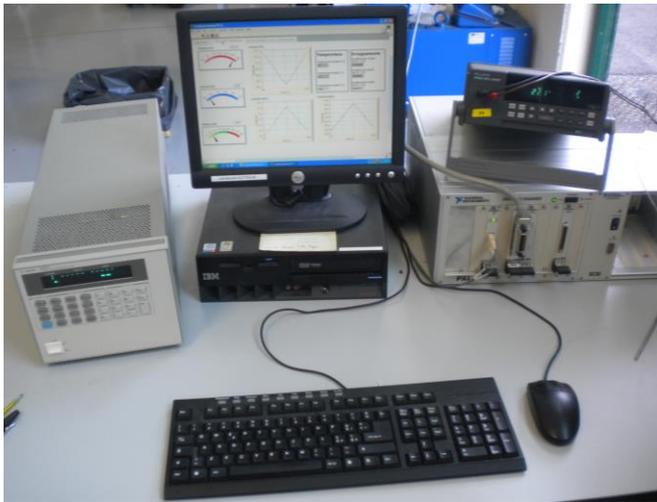
Figure 4. Electronic load, data logger, and host PC.
