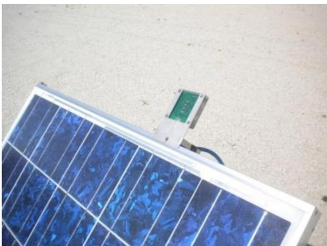
Figure 5. Sun metre mounted on the PV module.
