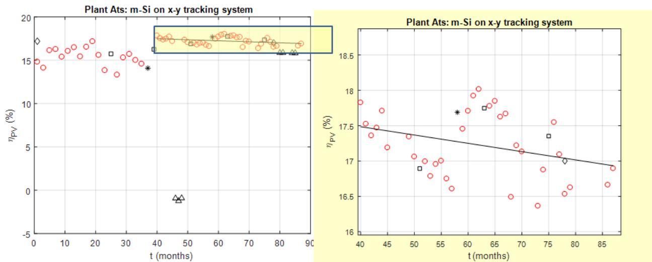
Figure 2. Estimated efficiency of plant  $A_{ts}$  based on m-Si PV modules on an x-y tracking system (red circles); black squares: values after adjustment of the monitoring system; black stars: values after module washing; black diamonds: values obtained by means of the capacitive load technique; black triangles: invalid data.
