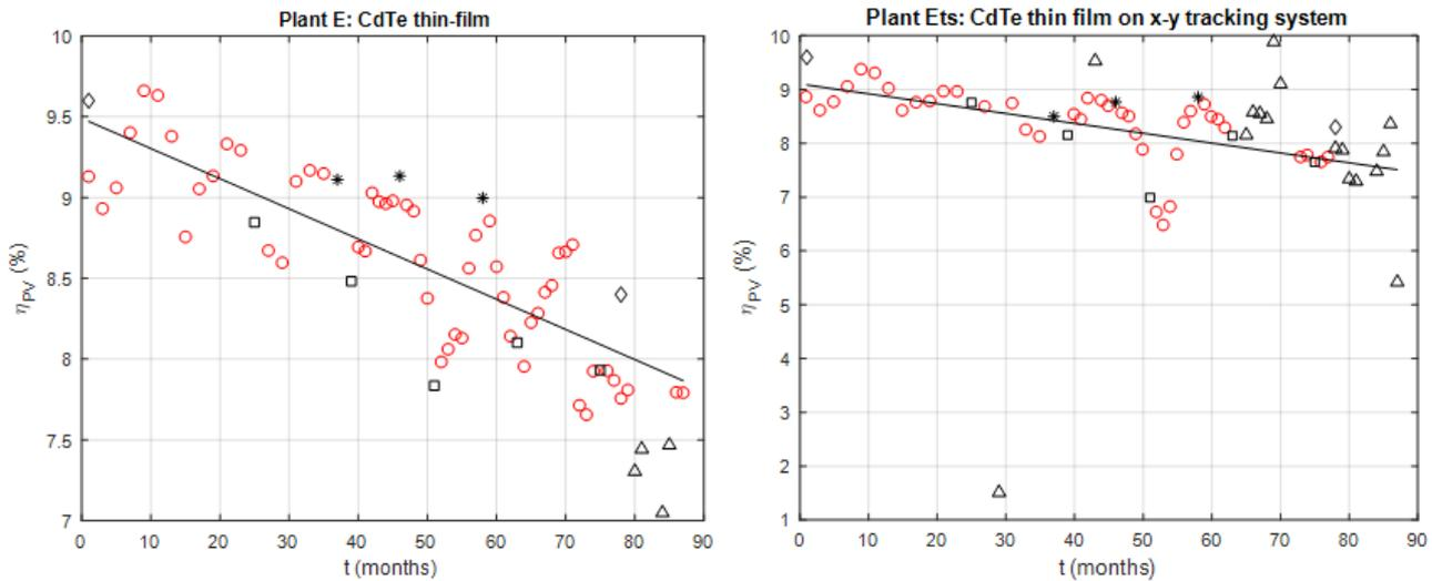
Figure 4. Estimated efficiency of the plants based on CdTe PV modules: E in fixed installation,  $E_{ts}$  on an x-y tracking system (red circles); black squares: values after the adjustment of the monitoring system; black stars: values after module washing; black diamonds: values obtained by means of the capacitive load technique; black triangles: invalid data.
