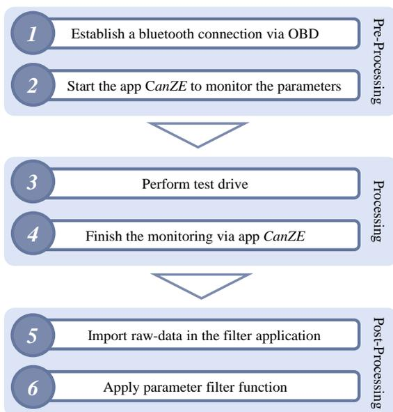
Figure 12. Procedure for acquiring structured driving data [24].
