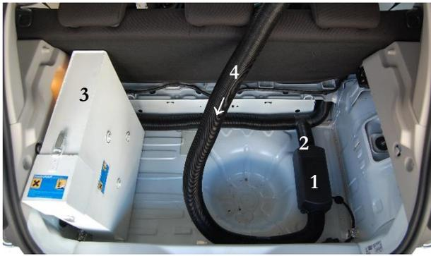
Figure 6. The assembled fuel-operated heater (1), air tubes (2), enclosed fuel tank (3), and fresh air intake (4) in the luggage compartment.
