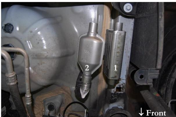
Figure 7. Partly mounted silencer (1) and oxidizing catalytic converter (2) for exhaust gases (view from below the floor panel).
