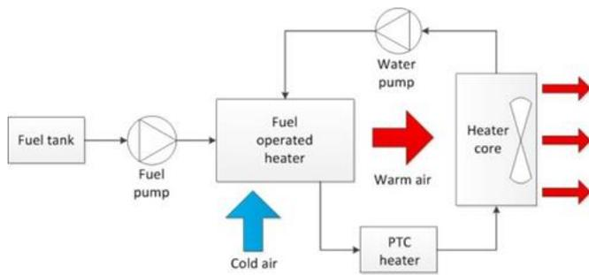
Figure 3. A water circuit incorporating a fuel-operated heater.
