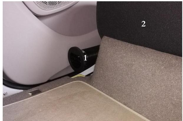
Figure 9. Front-facing hot air diffuser (1) on the right side of the backseat (2).
