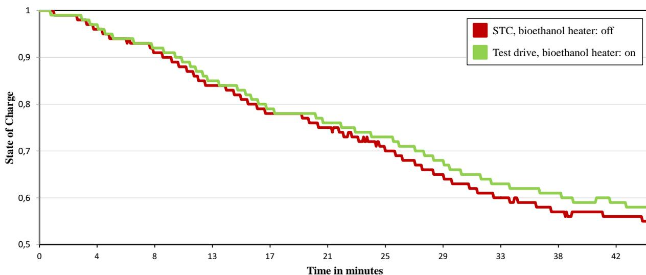
Figure 14. Comparison of the state of charge in two test drives at 1 °C; (SOC = 1: fully charged battery; SOC = 0: entirely uncharged battery).
