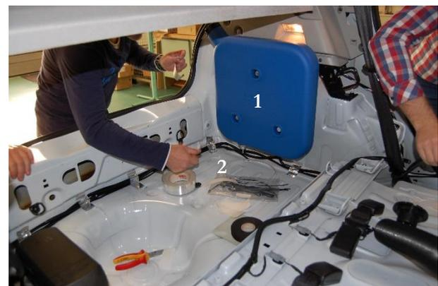
Figure 10. Fuel tank (1, without enclosure) as well as wiring and piping (2, not covered by interior trim) during installation and assembly.
