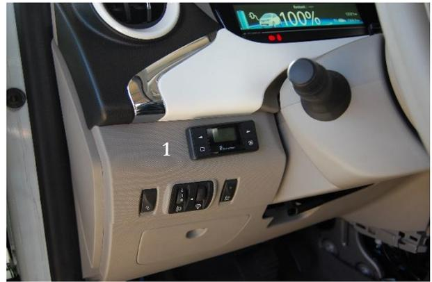
Figure 8. "EasyStart Timer" (1) mounted next to the steering column.
