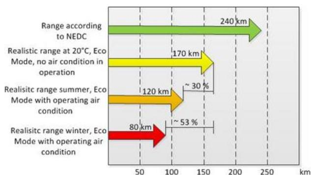
Figure 1. The range of Renault ZOE R240 according to [6].
