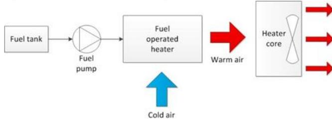
Figure 4. An air circuit incorporating a fuel-operated heater.
