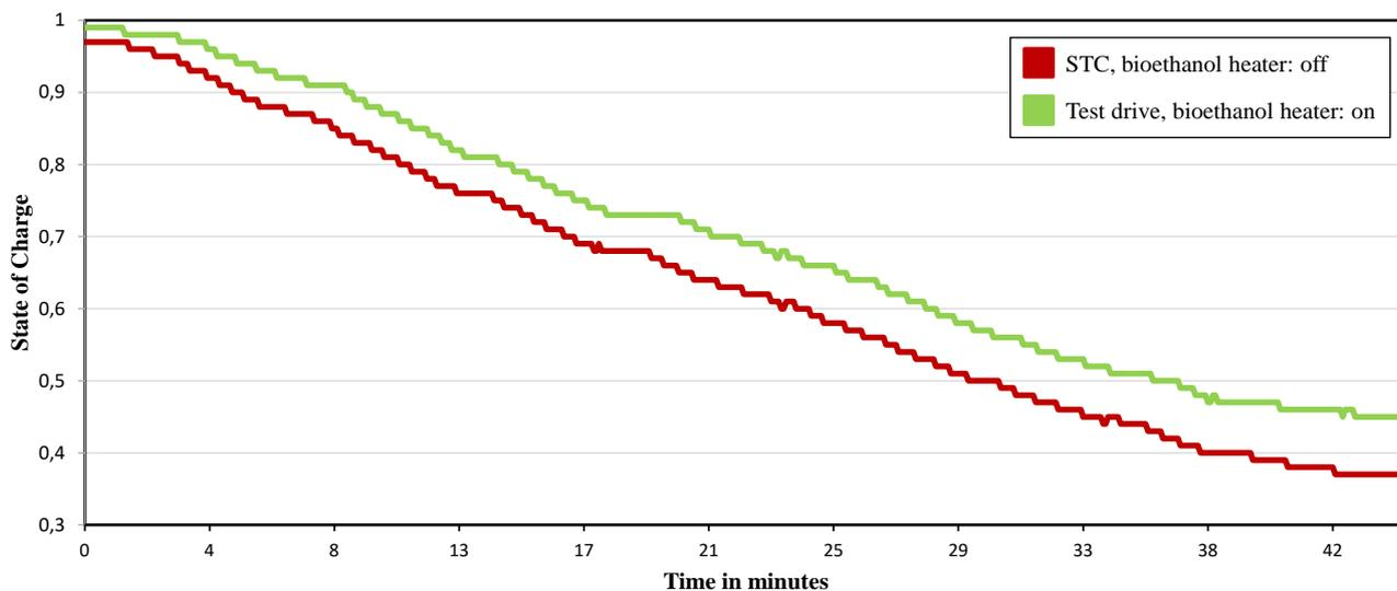
Figure 13. State of charge of two test drives at -11 °C (STC) and -13 °C (test drive); (SOC = 1: fully charged battery; SOC = 0: entirely uncharged battery).
