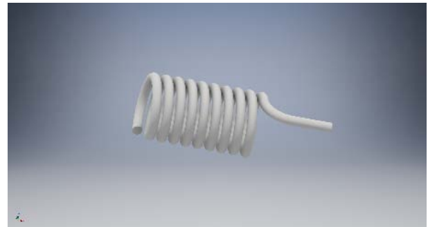
Fig. 2. CAD image of measuring end of thermometer
