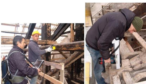
Figure 2 a) the GPR instrument (left); b) the Resistograph (right).
